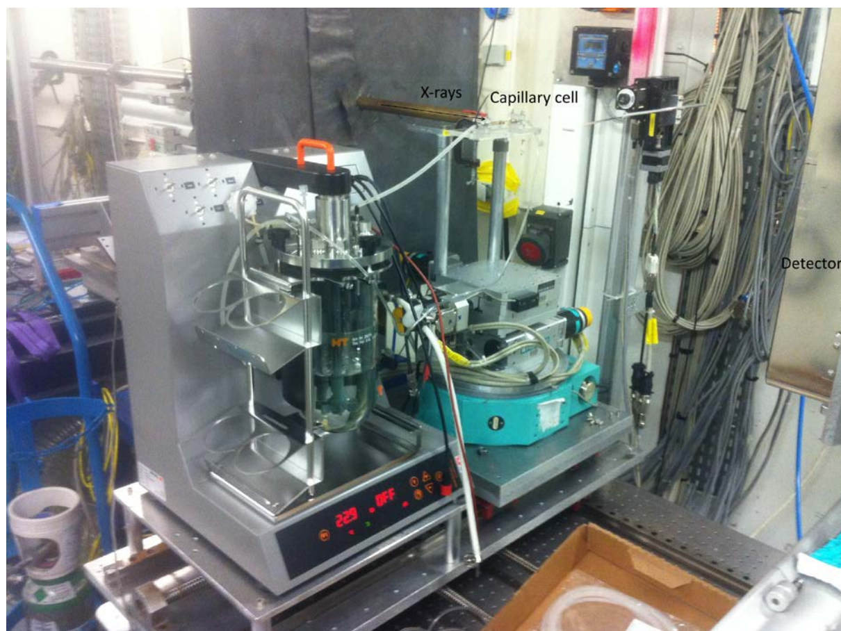
Figure 1. Minifors chemical reactor installed at beamline ID15B (ESRF) for high-energy X-ray diffraction experiments. The reactor is coupled to an observation cell. Credit: Alejandro Fernandez-Martinez.
