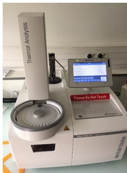
Figure 1: Left: General view of the TGA-DSC3+ instrument, with the cooling system (Minichiller, left down) and the gas entries (right side). Right: detailed view of the instrument, with the automatic sample changer (left column) and the touch screen (right).
