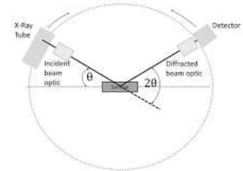
A typical powder diffraction setup
