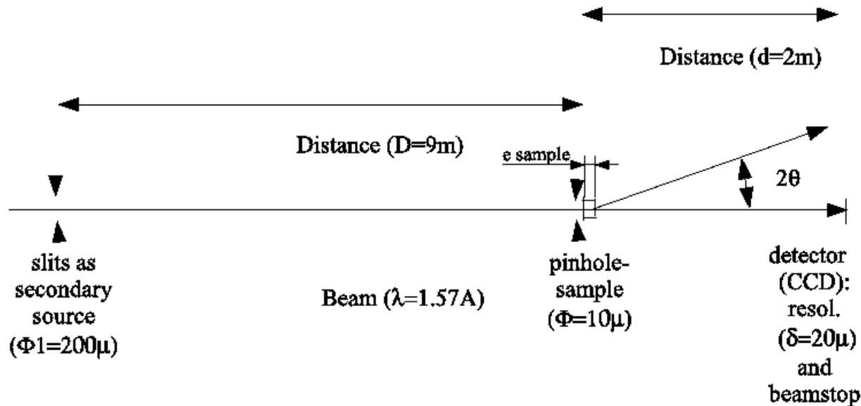
Experiments are similar to “Young’s hole” experiments which were used in optics before the occurrence of optical lasers. The esrf source is essentially incoherent. One selects an x-ray beam:
