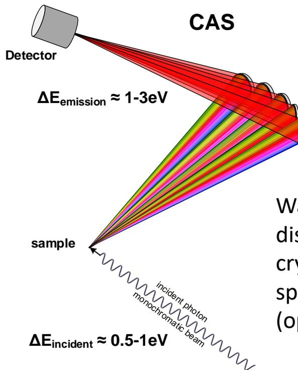
Wavelength dispersion with a crystal analyser spectrometer (optical)
