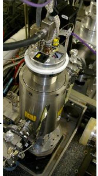
Example: liquid He cryostat → 4 K
